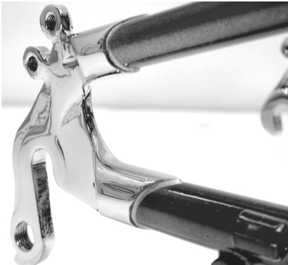
All Frames were fillet brazed by Hand in The ICE Workshops in Cornwall, England
