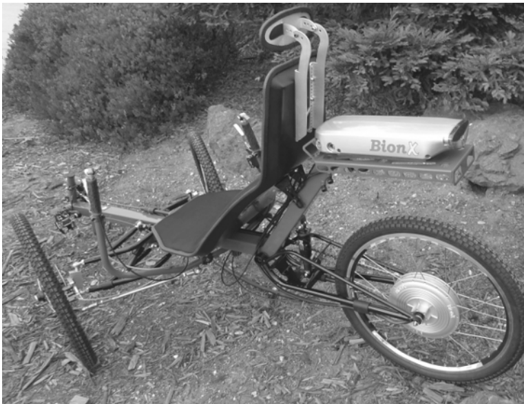
Berserker Tricycle Shown with hubcentric Bionx electric assist, and Rear Rack battery pack
